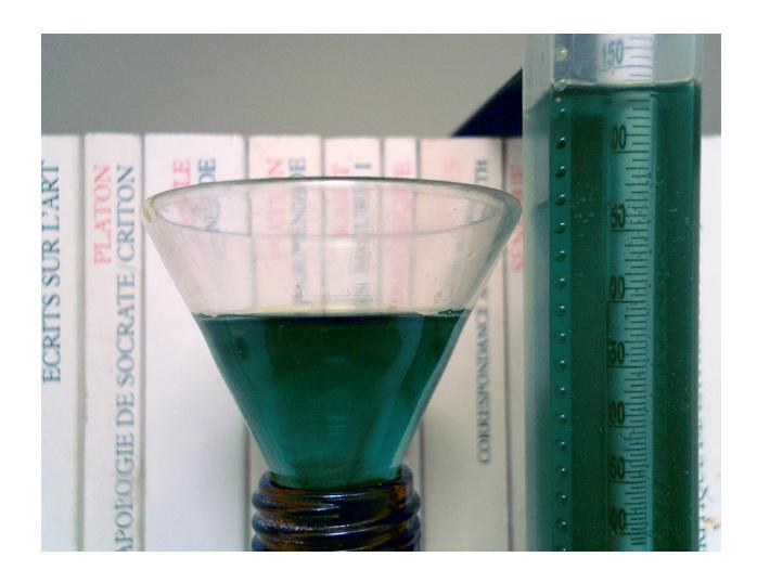
The simplest way of measuring this concentration is to use an aerometer as shown above.
